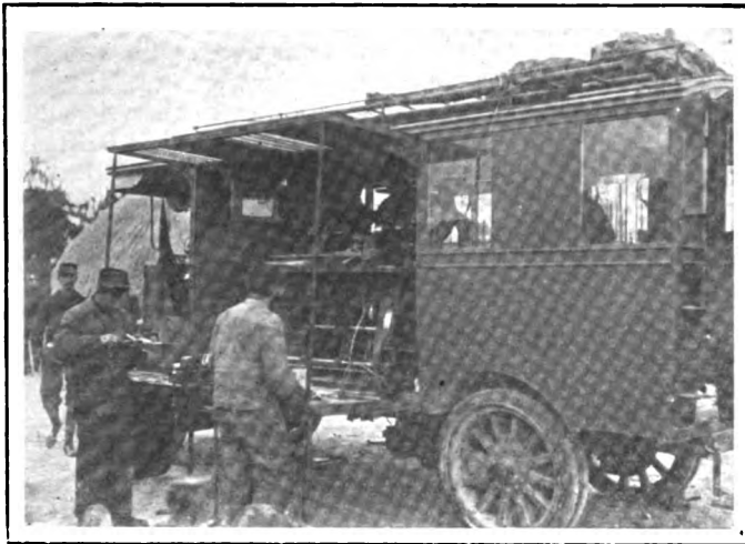
Portable wireless telegraph station used by the French army. This is a motor truck with a special body containing complete wireless outfit
